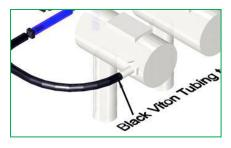
**Secure and route all tubing connections.** Take care to route the high temperature tubing away from the hot mufflers preventing chaffing/rubbing. Secure all tubing connections with a small zip tie. Heat shrink tubing also works very well!
