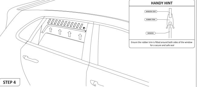
Roll up car window (WARNING if your car has a safety lock feature, do not roll window up all the way, ensure window is only just secured in bottom of rubber trim to avoid window automatically going down).
