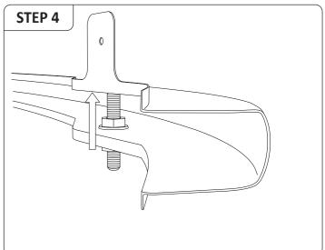
• Ensure the stud is flushed to the top section of the OEM Cross bar
