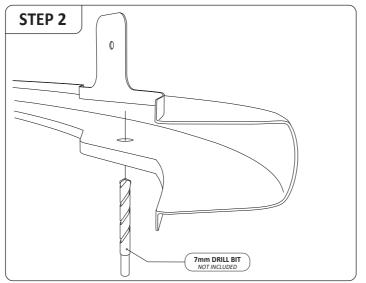
• Use a 7mm drill bit to enlarge the pilot holes to their final size.
