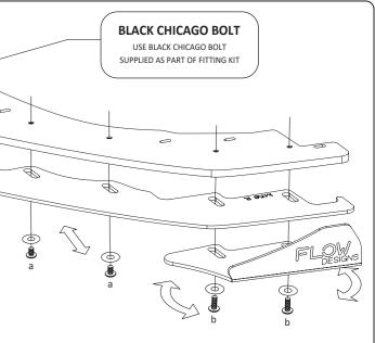
Insert bolts loosely into alocated brass thread locations. Slide and pivot extensions and winglets to your liking. • Use a 4mm hex key to hand tighten.
