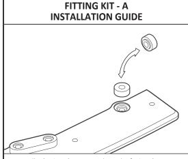
Install **3d printed spacer** with top lip **facing down** as shown in diagram above prior to installation of splitter. Push spacer into hole to lock into place.
