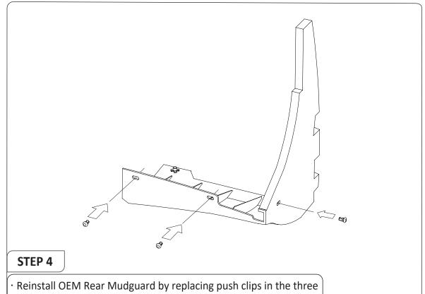
remaining holes not used by previously installed Jack Nuts
