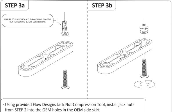
• Please ensure that the jack nut is firmly inserted into pre-drilled holes in OEM
