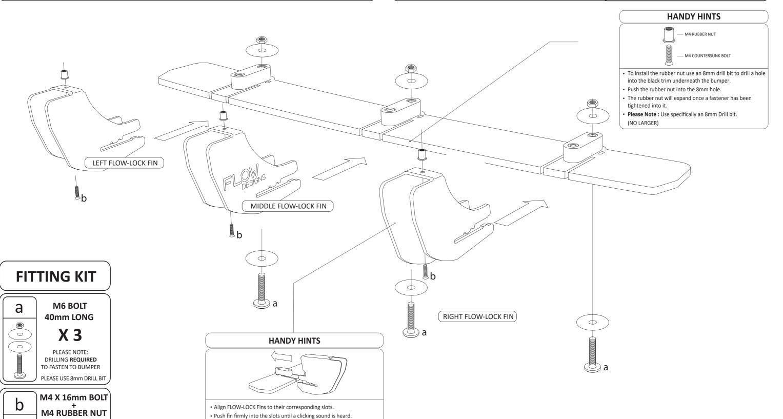
• Check both top and bottom locking tabs have securely seated. • Please ensure to allocate the correct FLOW-LOCK Fin to the correct
