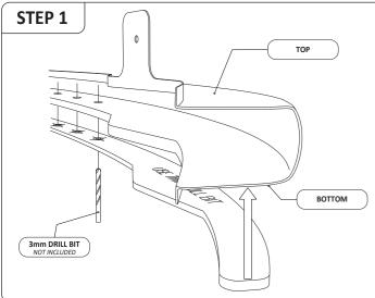
• Use a 3mm drill bit to drill 12 pilot holes into the cross bar.
