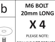
DRILLING NOT REQUIRED TO FASTEN TO SPLITTER DO NOT OVERTIGHTEN
