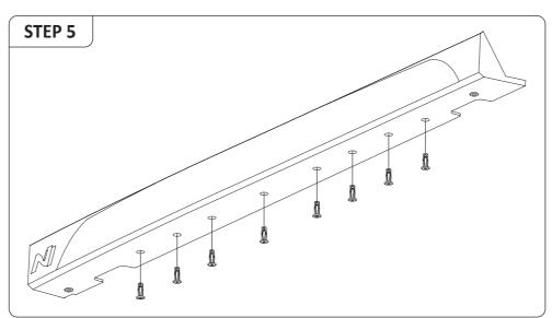
Using provided compression tool, install the remaining jack nuts into the OEM side skirt using the pre drilled holes
