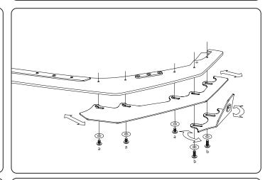
Insert bolts loosely into allocated brass thread locations. Slide extensions in and out to your liking.
