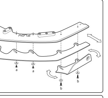
Insert bolts loosely into allocated brass thread locations. Slide and pivot extensions and winglets to your liking. • Use a 4mm hex key to hand tighten.
