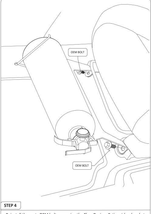
• Reinstall the seats OEM bolts, ensuring the Flow Designs Extinguisher bracket is also fastened
