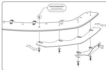
Insert bolts loosely into allocated brass thread locations. Slide extensions in and out to your liking. Use a 4mm hex key to hand tighten.
