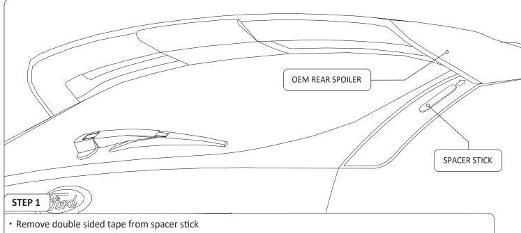
• Place the spacer stick on the rear tail light underneath the OEM rear spoiler by opening the boot. Ensure to place a spacer stick beneath both left and right tail lights.
