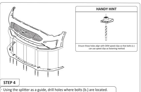
Ensure these holes align with OEM speed clips so that bolts (b.) can use
