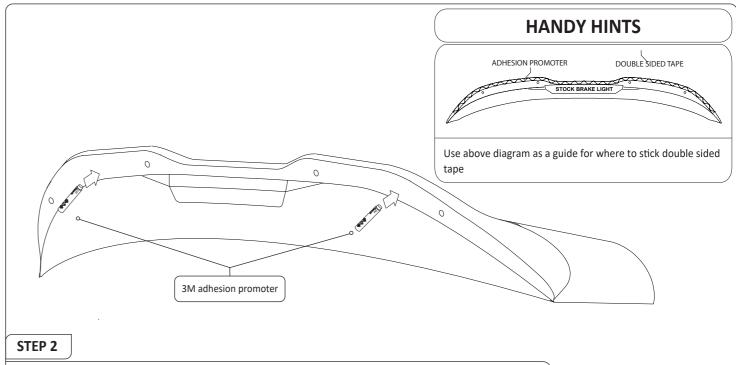
• Clean surface of OEM rear spoiler with alcohol swab, then apply 3M adhesion promoter to where double sided tape will be applied on OEM rear spoiler
