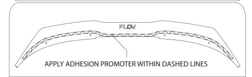
Use above diagram as a guide for where to apply the 3M adhesion promoter to the Flow Designs Rear Spoiler Extension
