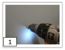
Drill an 1/8" Pilot Hole for Wood Installation.
