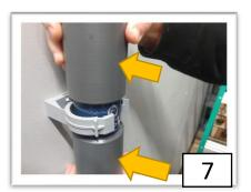
Press HD-9 Unit into Mounting Clamp until it latches in place.
