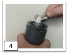
Thread ¼" Tube Fittings into each side of the HD Unit and use Wrench to tighten.
