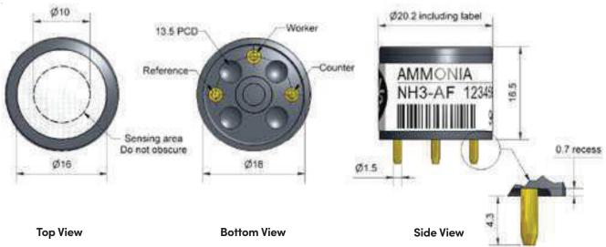
Dimensions are in millimetres (± 0.15 mm).
