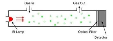
The basis of the NDIR technology is an infrared (IR) lamp that directs waves of light through a tube filled with a sample of air, toward an optical filter in front of an IR light detector. The IR light detector measures the amount of IR light that passes through the optical filter for the CO2 gas wavelength. The IR radiation produced by the lamp, includes the absorption band of CO2
