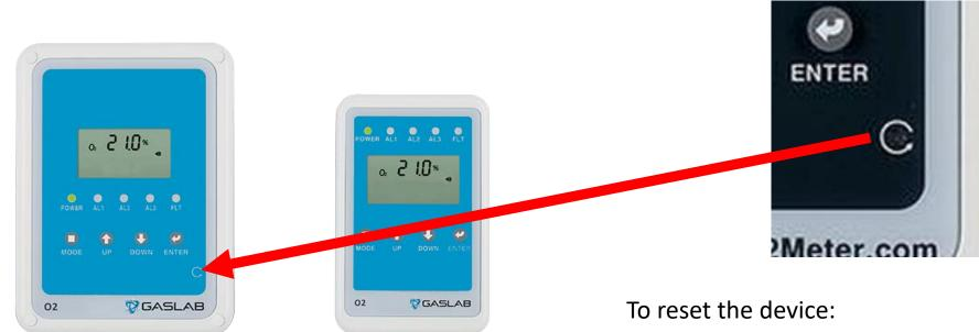
On the main unit in the bottom right-hand corner is a small hole with a white arrow circling it. Behind this hole is a soft, rubberized button.
