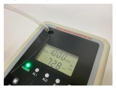
The device will begin to display increasing % values of O2 eventually driving the device in to all three alarm stages.
