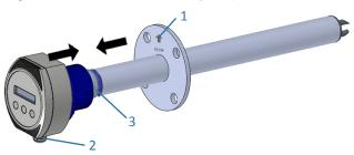
**7c.** Using a 10mm socket (or spanner) tighten clamp (3) to secure the head housing in position; torque to 5Nm.
