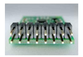
VCC = 5VDC. The analog output of the IAQ-2000 is specified for 0...5V corresponding to 350-2000ppm CO<sub>2</sub> equivalents.
