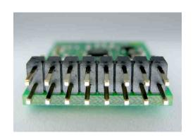
VCC = 5VDC. The  $I^2$ C-Bus, also called TWI-Bus (Two Wire Interface), allows reading the sensor prediction by  $I^2$ C-master. The  $I^2$ C functionality is optimized for a single-master system and can be implemented with the following parameters and addresses:
