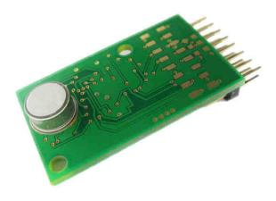
During the first 6 hours of continuous operation (burn-in) the module will display 350ppm, 2.5VDC, 50%PWM. The successful burn-in is saved to the EEPROM, the run-in time after restart is 15min.
