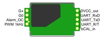
Figure 2. Diffusion Pin assignment
