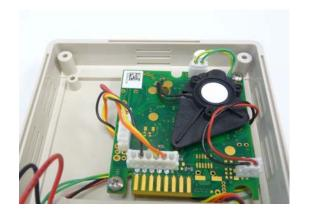
6. Gently take the filter, locate the vent and place the filter over the vent, covering the entire area.
