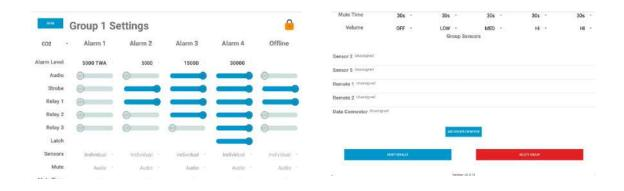
Each group features 4 configurable alarms. The alarm level, audiable on/off, Strobe, 3 realays, and latch setting are all configurable. The user can also deterimine if the alarms are to be triggered individually or if the entire grop is to be triggered. Lastly, mute settings and Factory reset can be found on this screen.
