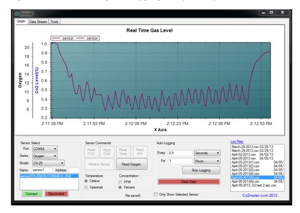
**Example 1:** Switch between nitrogen and oxygen gas every 2 sec. Cycles between 6-10% O2.
