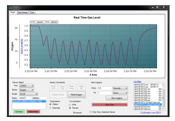
Example 2: Switch between nitrogen and oxygen gas every 5 sec. Cycles between 4-14% O2.
