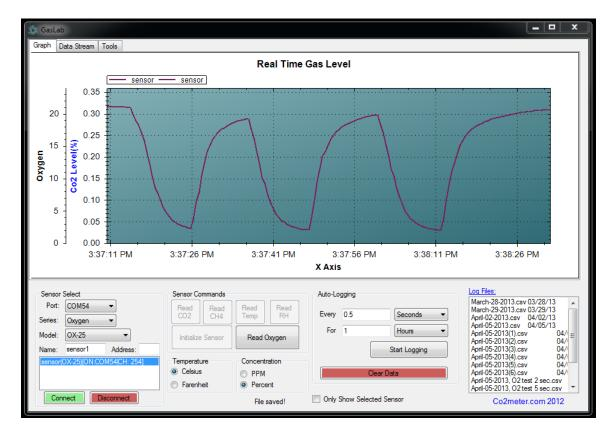
Example 4: Switch between nitrogen and oxygen gas every 15 sec. Cycles between 2-20% O2.
