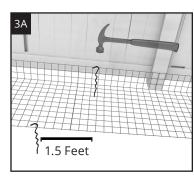
**3A.** Use a hammer to drive the provided 12" galvanized ground stakes into the ground ensuring that the hooked tip holds the wire mesh securely to the ground. It is best if the stake is positioned to hold the wire mesh where two strands of wire intersect. It is recommended that stakes are placed approximately every 1.5 feet (left to right) and alternated from front to back as shown. Additional stakes are available for purchase if needed.
