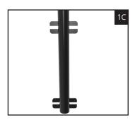
**1C.** The width of the mounting slots allows the use of fasteners up to 5/16" in diameter. For smaller diameter fasteners like wood screws, it is recommended that a washer be used under the head of the screw so that the washer + screw catches the face of the mounting brackets. The open slots of the mounting brackets allow a number of standard sized U-Bolts to strap the arms to round or square metal posts.
