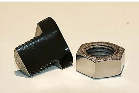
Milled surface on screw and nut.
