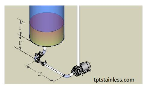
Suction restriction: DO NOT install any system throttling valves or similar devices to control the flow rate in the supply. Any system throttling valves or similar devices to control flow rate must be installed in the discharge line. Restriction in the supply line may cause cavitation and pump damage
