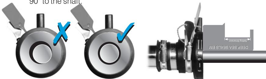
5. Check that the shaft is central to the sterntube, this ensures that the engine is correctly aligned and that the seal will run concentric to the shaft.
