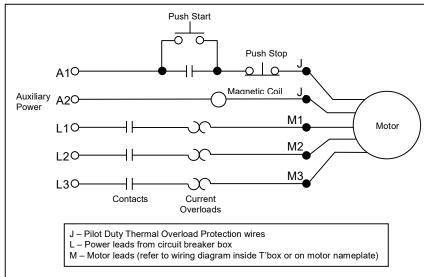
The schematic is shown for a three phase motor. For a single phase motor disregard L3 and M3. Pushing the START button completes the auxiliary control circuit, allowing current to flow through the magnetic coil. The contacts are magnetically closed, starting the motor and latching the auxiliary circuit. The motor will continue to run until the STOP push button is depressed, the motor reaches the overload temperature, or the current sensing overloads trip out.
