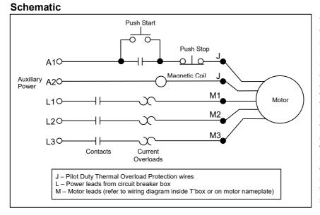
The schematic is shown for a three phase motor. For a single phase motor disregard L3 and M3. Pushing the START button completes the auxiliary control circuit, allowing current to flow through the magnetic coil. The contacts are magnetically closed, starting the motor and latching the auxiliary circuit. The motor will continue to run until the STOP push button is depressed, the motor reaches the overload temperature, or the current sensing overloads trip out.
