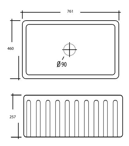
\* DUE TO THE MANUFACTURING PROCESS SINKS MAY HAVE SLIGHT VARIANCES IN SIZE. THESE DIMENSIONS SHOULD BE USED AS A GUIDE ONLY. WE STRONGLY RECOMMEND THE SINK BE ON SITE WHEN CABINETS OR BENCH TOPS ARE BEING PREPARED FOR THE SINK.
