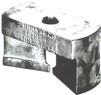
CAT. NO. 662-TMP-6D DOUBLE SECTOR FACE TAMPING HEAD —Two symmetrical sector faces each pi sq. in. (Test Method Tex-113-E) for use only with 6 in. ID molds. Attaches to tamping shaft of Automatic Tamper to form 10.0 lb. rammer. Machined ductile iron. 6 in. sponge rubber pad included. Approx. Ship. Wt.-9 lbs.
