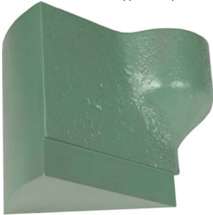
CAT. NO. 662-TMP-6S TAMPING HEAD —Machined pi sq. in. sector face for use only with 6 in. ID molds. Attaches to tamping shaft of Automatic Tamper to form 5.5 lb. rammer. Ductile Iron. Approx. Ship. Wt.-4 lbs.
