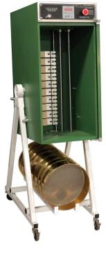
Note: for first time operation (or if the power has been interrupted, either by unplugging the sifter or a power outage), press the emergency stop button in; connect the power, then press the "Relay Reset" button in the top panel inside the cabinet. The sifter should operate normally.
