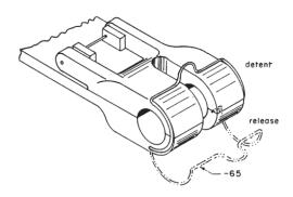
• Nylon sleeve bearings are wrapped off and on the shaft; their flanges contact the drive
