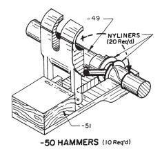
pin (which is straddled by the hammer). It may be necessary to replace the Nyliner bearings to provide perfectly free movement.
