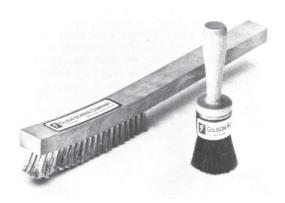
CAT. NO. RGTSA170 BRUSH, WIRE CLOTH (Bristle) – The round 1 ¼" dia. brush is a soft black bristle brush recommended for cleaning No. 16 and finer wire cloth. It has a nickel steel ferrule and clear lacquered handle. Overall length is 5-¾". Ideal for round sieves and pans. Also useful for screen trays. Approx. shipping wt:.2 lbs.
