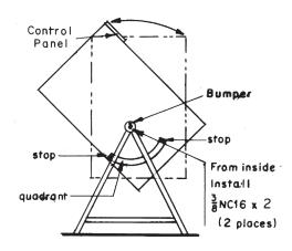
3) Install the two 3/8-in. dia. Capscrews from the inside of the cabinet by screwing them into the pivots at the top of the stand.
