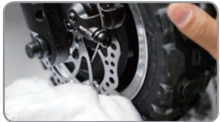
(4) Wipe the inner side of the disc while rotating the wheel
