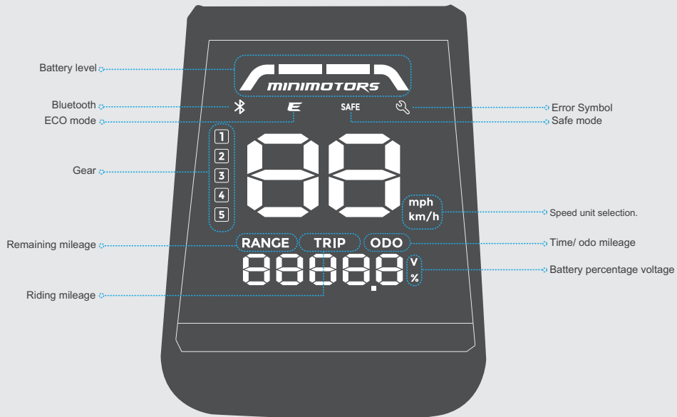
Minimotors EY2 smart digital screen (size: 47*50mm)
