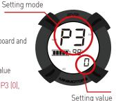
P PZ Speed unit 8(Fixed) 60(Fixed) 15(Fixed) O[Fixed] 0(Km/h), 1(mp/h) P9 Start method Cruise mode Slow start Max output Battery save Of Acceleration start). 0(0FF) 0(Off:Power 5~100% 1(MAX SAVE) start~5(Slow start) (User adjust) 1(Kick start) 1(0N) 2(MID SAVE) 3(NO SAVE) Pb Pd Electronic brake power LCD brightness control Auto off time setting ABS setting 0(Off)~5(Powerful) 0(Back light off)~5(Brightest) 0(OFF), 1(ON)
