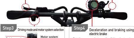
Set the use and strength of the electronic brake among the detailed functions of the instrument panel before driving. When the brake lever works, the electronic brake works together to increase the braking force.
