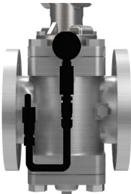
Thermal Relief Valve with Gauge A thermal relief valve releases thermal expansion inside the body to the line. It is combined with a gauge to check the pressure inside body.
