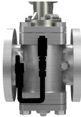
Thermal Relief to Body When the valve is closed, the thermal relief valve releases thermal expansion inside the body to the line.
