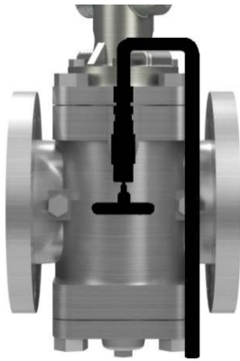
Manual Bleed Valve The simplest structure in bleed system. When the valve is closed, line leakage can be checked by bleed valve.
