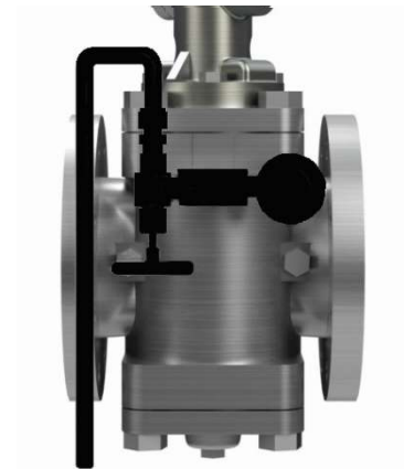
Manual Bleed Valve with Gauge A manual bleed valve is combined with a gauge. When the valve is closed, line leakage and pressure inside the body can be checked by bleed valve and gauge.
