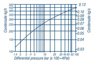
Note: Minimum Differential pressure for satisfactory operation 1.4 bar g with Positive Pressure and Discharge to atmosphere.
