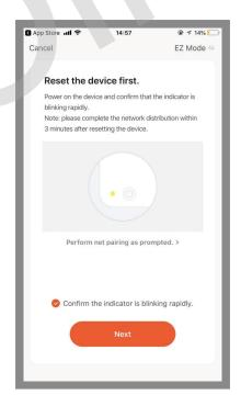
Step 5: Press and hold the controller WIFI learning button for 10s, WIFI blue light indicator is flashes, then check "Confirm the indicator is blinking rapidly" in the "tuya Smart" interface.
