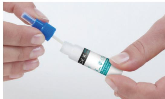
1. Take the bottle of super-plasticizer out of the pack. Unscrew the blue cap. Put the substance to be tested in the bottle and close it again. **Leave it standing (not horizontal) at room temperature overnight, or for about 12 hours.**
