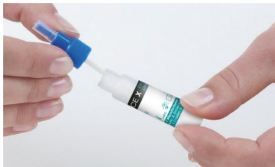
1. Take the bottle of superplasticizer out of the pack. Unscrew the blue cap. **Pour one to three drops of the suspicious liquid into the opened bottle.** Screw the cap back on and shake the bottle.
