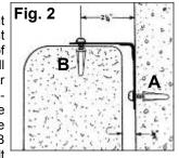
component C away from the wall to drill, molly and screw the bracket against the wall as shown in Fig. 2 (A). With bracket in place, reposition component C and drill, molly and screw the bracket to wall component Fig. 2 (B).
