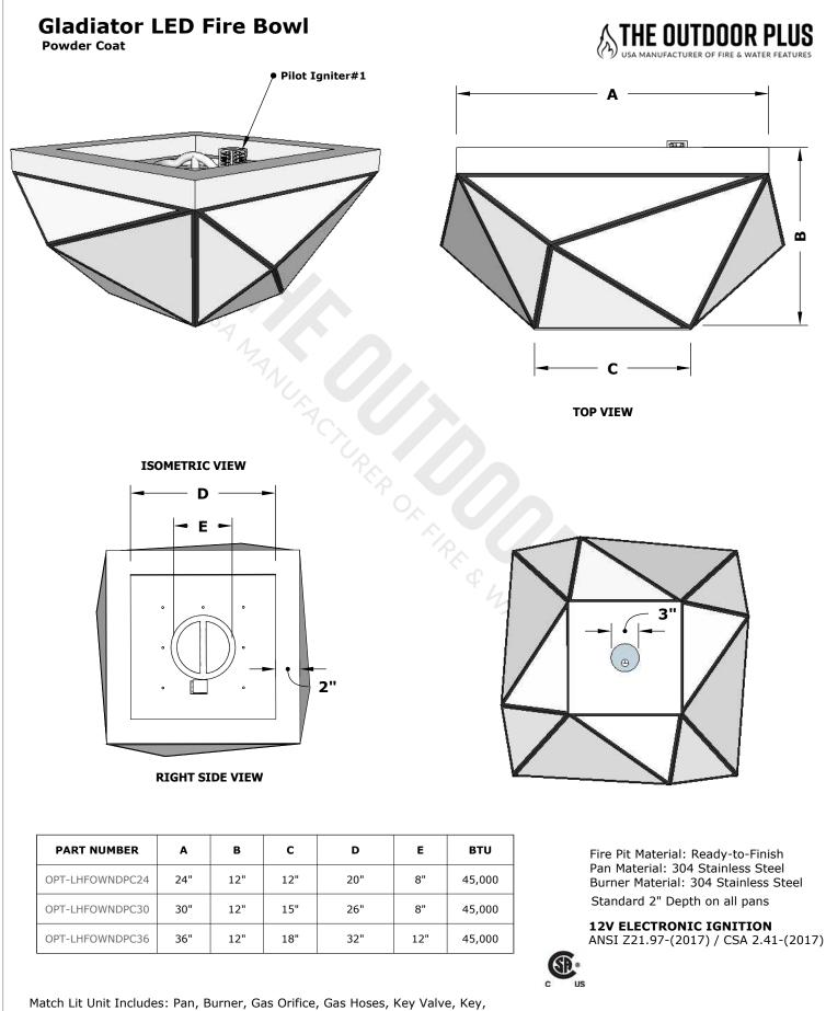
110v Ignition Unit Includes: Pan, Burner, Gas Orifice, Gas Hoses, Key Valve, Key, Plug & Play Electronic Valve, Pilot Igniter.
