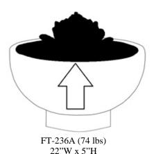
6. Holding the water feature disc (FT-236A) over the basin, insert the PVC connected to the non-kink tubing into the PVC coupling protruding from the bottom of the disc.
