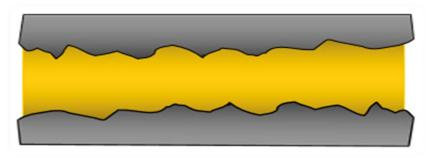
Full Film Lubrication: Full film lubrication, also commonly called Hydrodynamic lubrication, occurs when a robust lubricant film entirely separates the asperities of two surfaces. During full film lubrication, friction slowly increases as the load decreases and speed increases. Because hydrodynamic lubrication is associated with the least amount of wear, it is the most desirable
