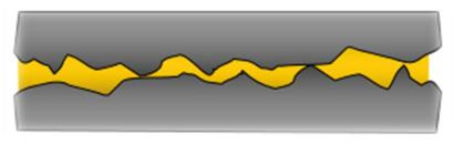
Mixed Film Lubrication: Occurs when components transition between boundary and hydrodynamic lubrication. A thin lubricant film between two surfaces leads to partial contact between asperities. The load is shared by both the lubricant and the surface contacts. As the speed increases or
